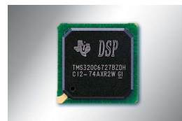
Tx/Rx DSP: TMS320C6727 Internal Clock: 250MHz 32-bit floating point Floating point calculation: 1800MFLOPS
