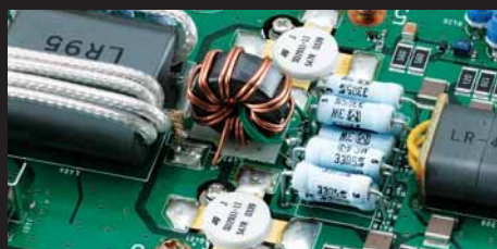
PA unit (close up)
